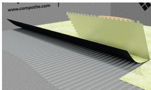
(only needed for waterproofing) After installing the sealing membrane, apply the seam tape and corners and continue according to the installation instructions of sealing products. Please use 5" PE seam tape on joints and all corners. Use 5" PE seam tape or you can cut 5" strips to make your own seam tape, seam is applied using thin set (Seam tape is non adhesive).
